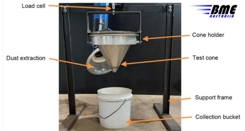
Figure 2. Flow rate test apparatus.
